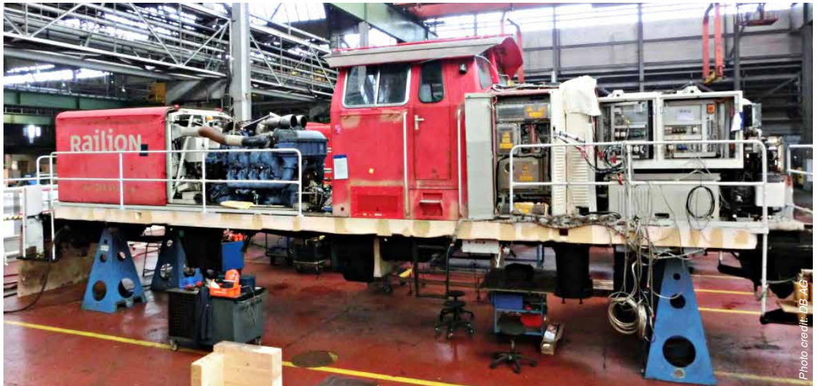
Switching a DB Cargo diesel shunting locomotive BR 294 over to a diesel/battery hybrid drive at the Cottbus depot – installation of the hybrid block
