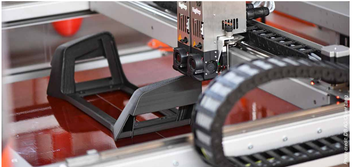
3D printing: producing a headrest
